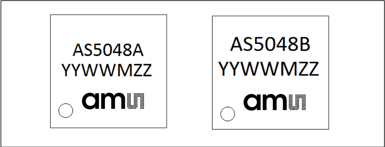
Figure 39: Package Markings for AS5048A & AS5048B
